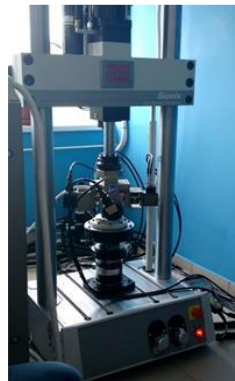
Hip prosthesis wear simulation
